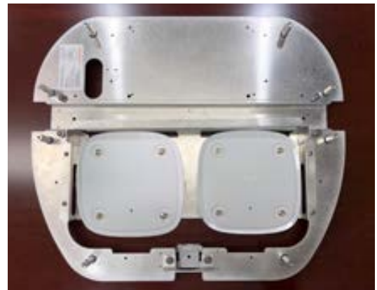
FIGURE 6: AP Installed on Frame
