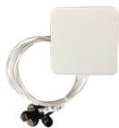
5 GHz Patch 6 dBi HBW:55 VBW: 60 Wall/Mast/ Pole TESSCO No 215098
