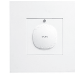
Ceiling Tile Enclosure Lightweight, powder-coated aluminum enclosure conceals and protects access points in suspended ceilings. Meets NEC300-22 and 300-23 for installation in plenum/air-handling areas.
