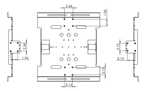
All holes have ¼-20 inserts. 1.96 x 2.36 hole pattern is for the omni antenna brackets. The 2.13 x 2.13 hole pattern fits the TerraWave Universal Articulating Mount, the optional TerraWave Industrial Articulating Mount and the optional Patch Antenna Paddle.
