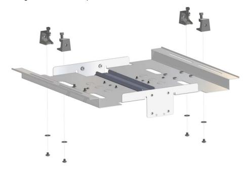
4A) Cisco APs: Attach the bracket supplied with the AP using qty 4 screws #8-32.
