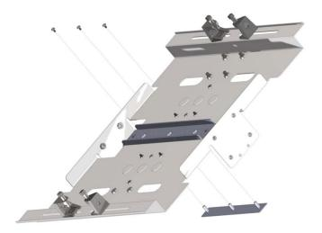
5) Bracket assembly can be installed vertical or horizontal. Slide I beam clamps to engage I beam and hand tighten I-beam bolts. Once bracket is centered, tighten I beam bolts with a wrench.
